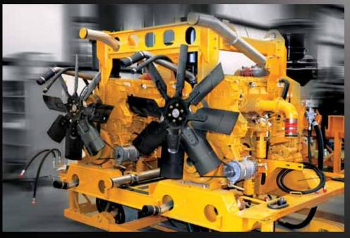
The T1655 features two CAT C18 ACERT engines for a total of 894.8-kilowatts (1200 hp). The dual engine configuration provides power to a common pump drive so that each engine provides full power to the machine. In addition, if one engine is not operational, the machine is still able to function on a single engine. The large 3028.3-liter (800 gal) fuel tank provides 13.2 hours of continuous operation at maximum horsepower.
