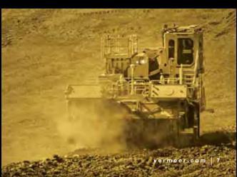
An air-ride suspension system on the cab provides a smooth, quiet ride for the operator in the typically harsh environment of a surface mining operation making the T1655 a comfortable machine to operate.
