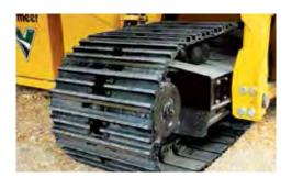
**SMART TRACK.** Control system monitors elevating face pressure and slows or stops the ground drive when the face pressure reaches a programmable level, reducing operator interface and increasing productivity.
