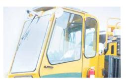
CAB. Designed for operator comfort, cab features include fully adjustable air-ride seat, cab pressurization with self-adjusting climate controls and large windows for excellent visibility.
