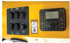
**JOBSITE EFFICIENCY.** Advanced Control System (ACS) controller monitors engine rpm and slows or stops the ground drive when it reaches the programmable set point to reduce stalling the turner in the windrow.
