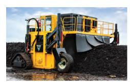
**CONVENIENT REAR CURTAIN.** Rear curtain is controlled from the cab and can be lowered to control windrow material deflection when entering a windrow. It can also be strapped down for easier transport.
