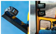
EASE OF OPERATION. New control display with a full instrument panel makes it convenient to read gauges at a glance — as well as see the sides and rear of the machine on the color display through the mounted rear view cameras.
