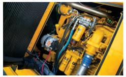
QUIET, EFFICIENT ENGINE FAN. Flexxaire fan pitch is variably adjustable, automatically reading the engine temperature and adjusting itself as needed, reducing horsepower consumption. Reversible to blow debris off screen.
