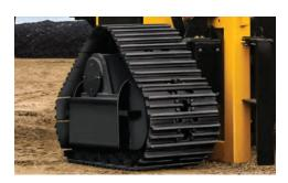
**CONQUERS YOUR TERRAIN.** When equipped with the independent two-wheel drive short track system, the CT718 offers improved traction in difficult composting sites.
