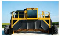
TRANSPORTABILITY. Machine height is 12.5' (3.8 m) for easier transportability. Ladder folds out for climb access and folds in to make the machine narrower for transport.
