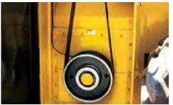
**RELIABLE COMPONENTS.** The poly-synchronous belt drum drive has proven to be a reliable system requiring little maintenance and offering adjustable shafts.
