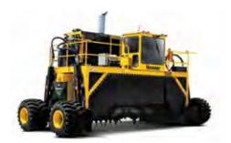
**EASE OF MAINTENANCE.** All grease points are accessible from ground level. Hinged, lockable doors on both sides of the engine provide spacious access for maintenance.
