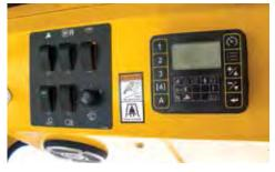
**JOBSITE EFFICIENCY.** Advanced Control System (ACS) controller monitors engine rpm and slows or stops the ground drive when it reaches the programmable set point to reduce stalling the turner in the windrow.
