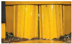
SMOOTH FEEDING. Vertical feed rollers with helical cleats help hold material firmly to the infeed table, which reduces vibration, shock and structural loading to the rear of the machine.
