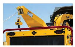
**EASILY LIFT HEAVY MATERIAL.** An optional winch allows operators to move large logs effortlessly. The 150' (45.7 m) winch line has 2000 lb (907.2 kg) pulling force and can automatically lift the log onto the feed table. With the chain choker detached it is also more easily attached to log than hook-on cable designs.
