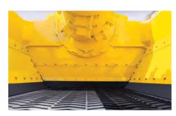
**HIGH PRODUCTION.** Designed to handle more production with less clogging, the 36" (91.4 cm) wide continuous undermill conveyor system offers optimum speed and capacity.
