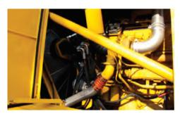
**ENGINE POWER.** A CAT C27 Tier 4i (Stage IIIB), Twin Turbo engine provides 950 hp (708 kW) of power to meet your jobsite demands.
