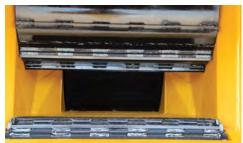
OFFSET HORIZONTAL FEED ROLLERS. The offset horizontal feed rollers are designed to efficiently take on oversized, branchy limbs.
