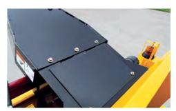
OPTIONAL WINCH. The 150' (45.7 m) winch line has a pull-in force of 3250 lb (1474.2 kg), making it easy to lift logs directly onto the feed table. The winch boom can be removed and installed conveniently with just six bolts. By removing the winch boom, the operator can mechanically feed the chipper more efficiently.
