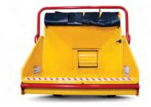
**LARGE INFEED OPENING.** The BC1000xL features a 12" (30.5 cm) tall and 17" (43.2 cm) wide infeed opening. This design can help boost productivity by decreasing the amount of trim cuts needed prior to processing.
