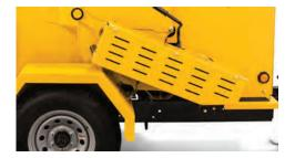
**CLUTCHLESS PTO.** The throttle integrated with the belt drive engagement process helps ensure that the PTO can be engaged only while the engine is at low idle/low rpm. Automatically, the engine throttles up to full rpm after the belt drive is fully engaged. This system helps to reduce premature wear to the belt drive system by preventing high idle engagement of the cutter drum.
