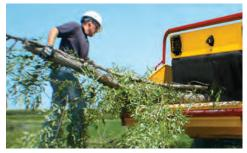
**SMARTFEED.** A patented feed-sensing control system that monitors engine rpm and automatically stops and reverses feed rollers when feeding large, hardwood material. With a simple switch, an operator can choose between three rpm droop settings to fit the specific job application.
