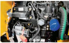
**ELECTRONIC FUEL INJECTION (EFI) ENGINE.** An 89 hp (66 kW) Power Solutions International (PSI) 3.0L EFI gas engine performs well during cold-weather starts, and provides improved fuel economy over comparable carbureted gas engines and increased/faster engine response under load.
