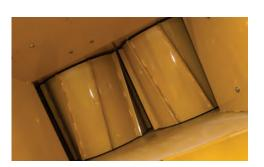
**SMOOTH FEEDING.** Vertical feed rollers with helical cleats help hold material firmly to the infeed table which reduces vibration, shock and structural loading to the rear of the machine.
