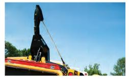
**OPTIONAL WINCH.** Eliminates the need to drag large material to the chipper. The 150' (45.7 m) winch line can handle material up to 4000 lb (1814.4 kg), making it easy to lift logs directly onto the feed table. In addition the winch can also be hydraulically raised out of the way to allow operators to feed the unit using a loader.
