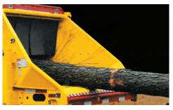
**SMART CRUSH.** Once the upper feed roller freely raises for four seconds, it will automatically increase down pressure on the material being fed. This allows the upper feed roller to easily climb onto large forked material before the increased down pressure is applied for maximum pulling force.
