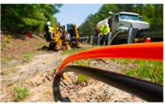
CLASS-LEADING CYCLE TIMES. The D40x55 S3 features a carriage speed of 188 ft/min (57.3 m/min) — which is 7% faster than its predecessor, the D36x50 Series II — helping contractors install more linear feet per day.
