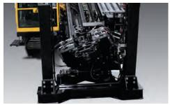
**OPEN-TOP VISE.** An angled, open-top vise allows for the passage of larger tooling. Because of the large opening, operators can also use it to break out tooling.
