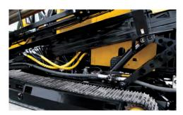
INCREASE YOUR RANGE. Unique four-bar linkage rack and additional pads allow operators to set up entry angles of 11° - 24° — increasing range attainable with tracks fully on ground.
