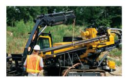
KNUCKLEBOOM CRANE. The optional knuckleboom crane mounted on either side of the base anchor maneuvers heavy tooling, reducing the need for support equipment.
