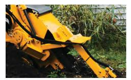
MAKE SENSE OF YOUR TRENCH. When difficult conditions are encountered while trenching, causing a sudden drop in engine speed, the TrenchSense<sup>™</sup> electronic control system automatically pauses the forward motion of the tractor to prevent engine shutdown and recalibration of the machine controls. Once preset engine and trencher speed recovers, forward AutoCreep resumes. The sequence occurs within seconds and requires no operator adjustment.
