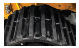
**QUAD TRACK SYSTEM.** The quad track system offers improved floatation, reduced surface damage and increased tractive effort. Four-wheel steer and crab steering are functional with both quad track and tire options.
