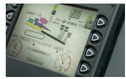
MAKEUP OR BREAKOUT. Controls provide options including automated sequence, partially automated sequence or manual sequence of the rod makeup/breakout process, depending upon operator preference and level of expertise.
