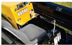
**OPERATOR'S STATION.** The D6x6 has dual axis control valves. Vise controls are integrated into the right- and left- hand joysticks. With this design, the operator's hands do not have to leave the joystick to run the controls.
