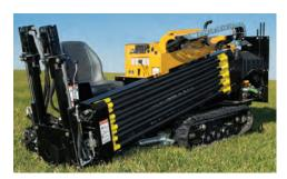
POWER-TO-SIZE RATIO. The D6x6 has the most compact footprint in its class of horizontal directional drills. With a 25 hp (18.6 kW) engine, the unit has 550 ft-lb (745.7 Nm) of rotary torque and 5500 lb (2494.8 kg) of thrust/pullback.
