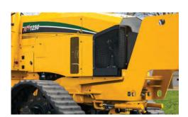
INCREASED POWER. When the RTX1250 engine drops from 2500 rpm to 2300 rpm under load, the horsepower increases from 120 hp (89 kW) to 127 hp (95 kW), allowing the ride-on tractor to run at maximum horsepower in work mode.
