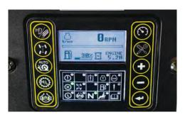
KNOWLEDGE ON DISPLAY. An integrated display allows the operator to optimize machine performance by adjusting operating attachment and ground drive parameters using machine diagnostic information — including engine rpm, fuel level, battery voltage, engine coolant temperature and engine hours.
